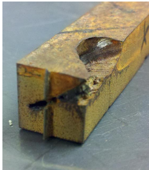
Figure 10: Boiler plate surface gash
