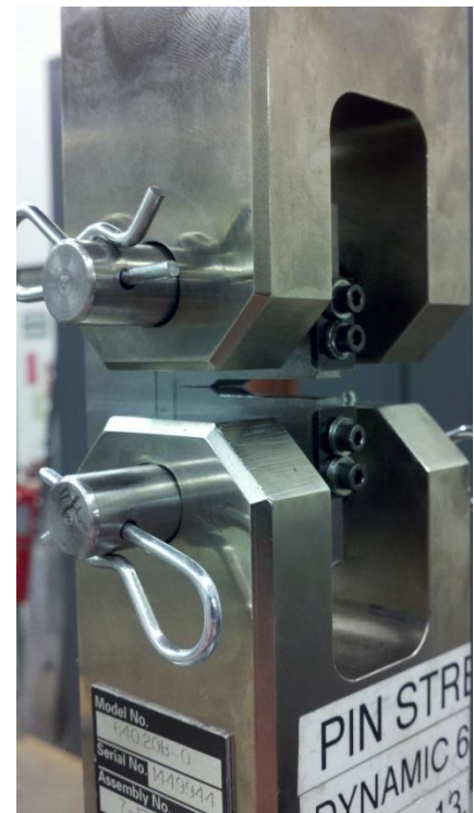
Figure 2: Fracture toughness testing setup
